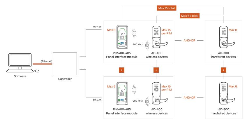
AD-400 wireless range up to 200' in typical building construction, up to 1000' line of sight.
