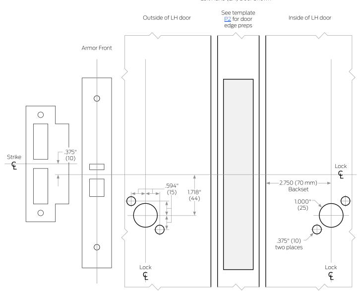
Refer to Template P1 for case and strike dimensions and if applicable information to prepare the door for wire routing. Armor front deadbolt, auxiliary latch and latchbolt holes shown for dimensional purposes only. Use door edge measurements for door preparation.
